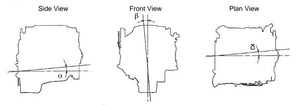
Figure 3.3.4.2 Installation Angles
